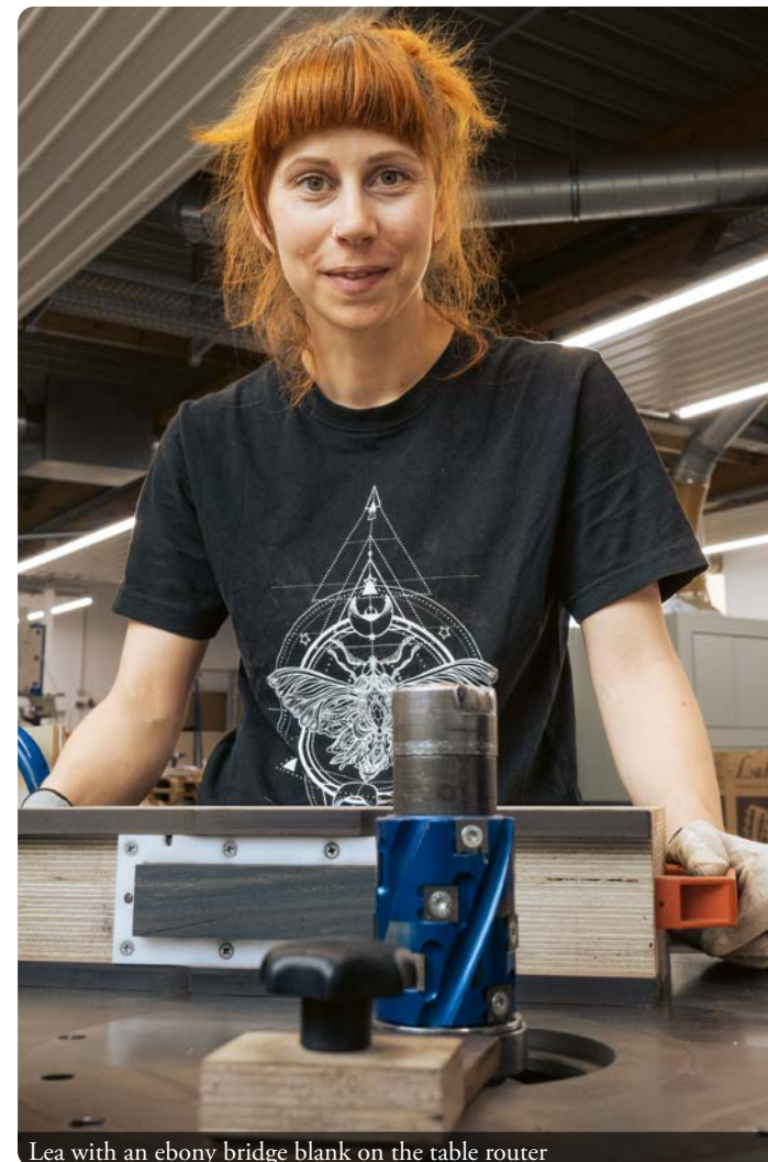
Lea with an ebony bridge blank on the table router
