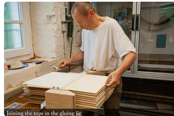
Joining the tops in the gluing jig
